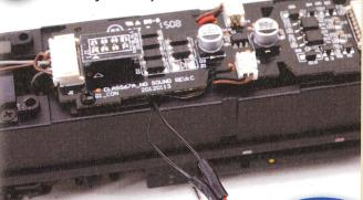
Finally, the 8-pin plug of the TTS decoder was plugged into the socket, ensuring the orange wire lined up with Pin 1, and the decoder was prepared for final installation by covering one side with electrical insulation tape. This will be used to fix it to the roof of the Class 67 body during reassembly.
