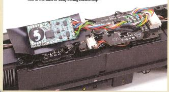
Speakers make a tremendous difference to the sound output of a decoder and there are plenty to choose from. Be sure to check that the specification of the speaker and decoder will match otherwise you could damage components on the decoder.
